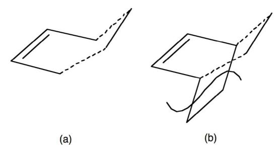
• the next step is to set the interfragment distances (dashed lines in (a) above ) to a value appropriate to the TS. For a percyclic reaction, the partly formed  $\sigma$  C-C bonds in the transition state are around 1.9 to 2.3 Å. It is suggested that you use a distance of 2.1Å.
