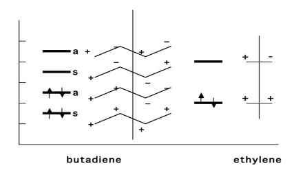
The HOMO of ethylene and the LUMO of butadiene are both s (symmetric with respect to the reflection plane) and the LUMO of ethylene and the HOMO of butadiene are both a. Thus it is the HOMO-LUMO pairs of orbital that interact as shown in the following diagram.
