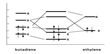
The important point is that it is the HOMO of butadiene (a) that interacts with the LUMO of ethylene (a). The HOMO of the adduct is thus a.
