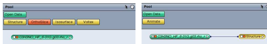
Fig. A.2 Initialization of Avizo STR module. Left: Green box with the electron density grid data. Right: Creating yellow box with the structure data for the oxazole molecule
